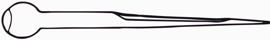
B. Closed spear for sampling small grains such as wheat.
